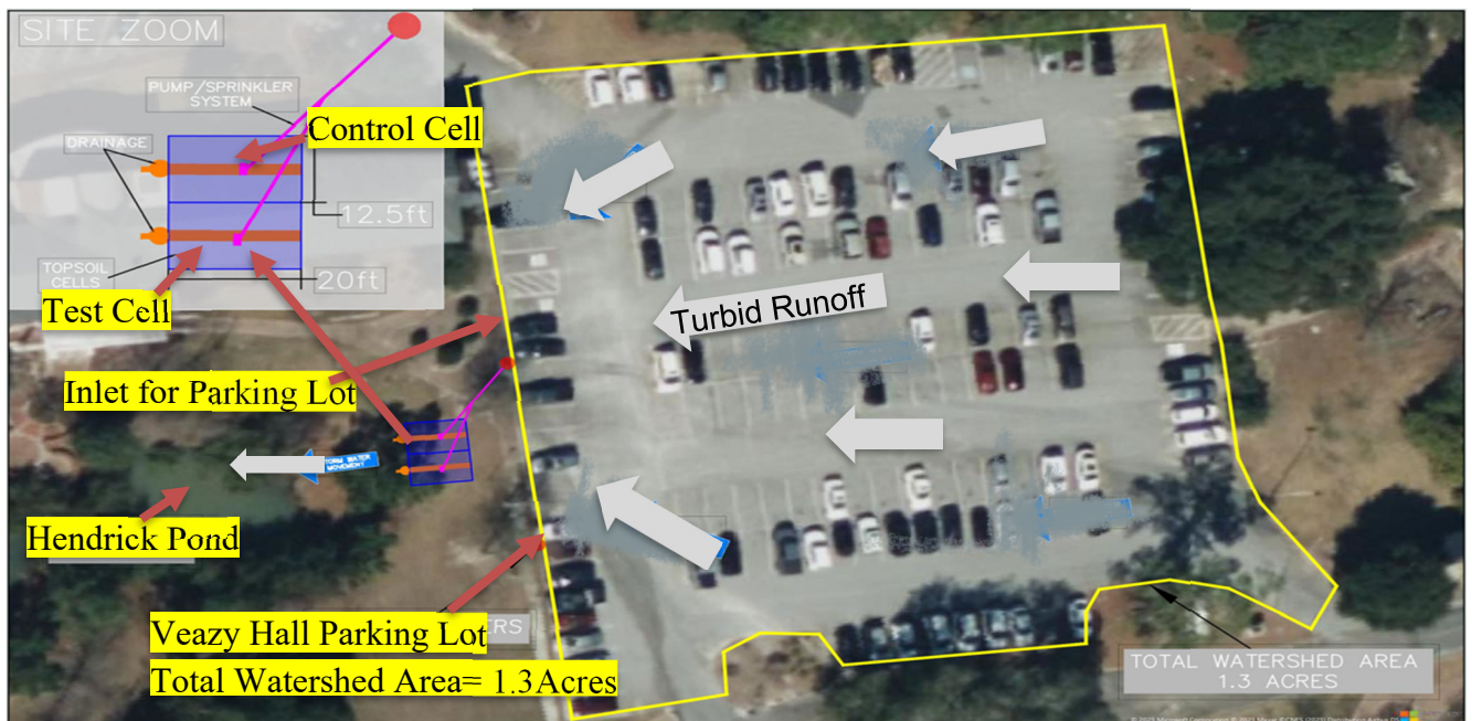
Figure 7. Full-Scale Field Test Site for On-Site Treatment of Stormwater Runoff from Veazy Hall Parking Lot (GSU Campus)
