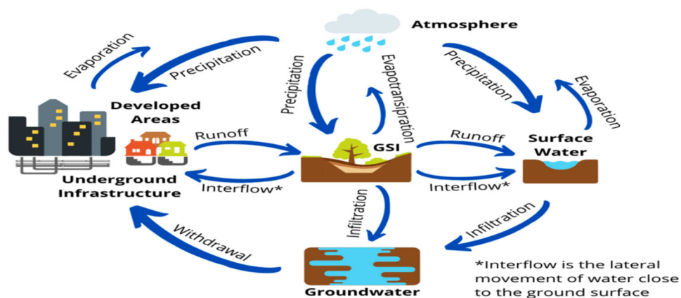
Figure 1. Conceptual diagram of water flow paths in the context of GSI (Taguchi 2020)
