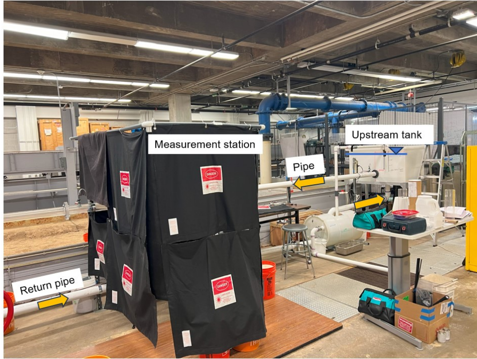
Figure 1: The reservoir-pipe-reservoir system used in this study.
