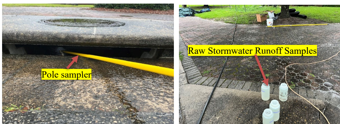
Figure 23. Raw stormwater runoff sampling at the Inlet for Parking Lot
