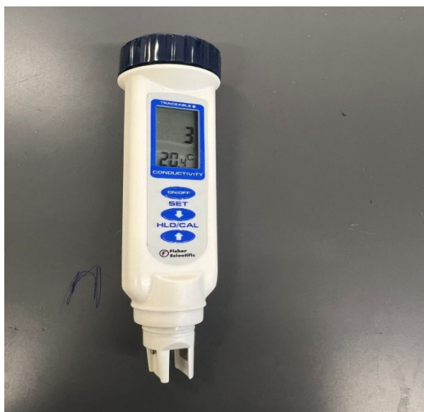
Figure 28. Fisher Scientific Traceable Conductivity/TDS Pocket Tester
