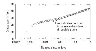
Figure 3. Drawdown as a function of log time in well 33P030 at a pumping rate of 552 gallons per minute, Fort Stewart, Georgia, April 26, 2010.
