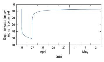
Figure 4. Measured water level in well 33P030 during a 24-hour aquifer test, Fort Stewart, Georgia, April 26–May 3, 2010.
