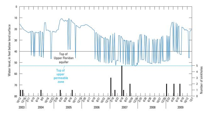
Figure 3. Water-level measurements in well 12L382 with respect to depth to the top of the Upper Floridan aquifer and the top of the upper permeable zone and number of sinkholes reported during October 2003–December 2009. See Figure 4 for well location.
