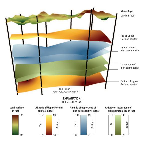
Figure 2. Three-dimensional geologic diagram of the well field. Space was added between each layer for visibility.
