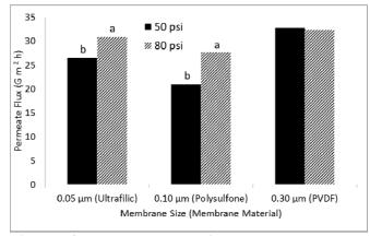
Figure 4. Poultry processing wastewater mean permeate flux values (Gm<sup>2</sup>h) for 3 filtration membranes at 50 and 80 psi
