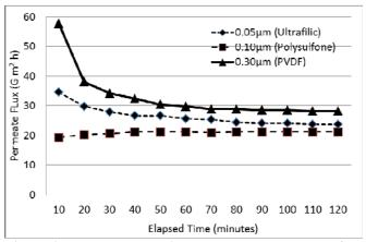
Figure 2. Poultry processing wastewater permeate flux  $(G m^2 h)$  values at 10 minute intervals for 3 membrane filters at 50 psi operating pressure
