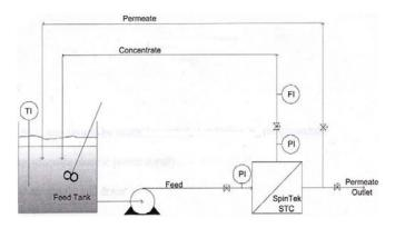
Figure 1: Spintek Static Test Cell (STC) Membrane Filtration System (Source: http://www.spintek.com/stc.htm)
