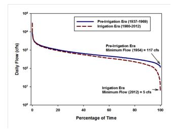
Figure 2: Comparison of flow duration curves for the pre-irrigation and irrigation periods of record at USGS gauging station 02353500 in the Ichawaynochaway Creek watershed (see Fig. 1 for location).
