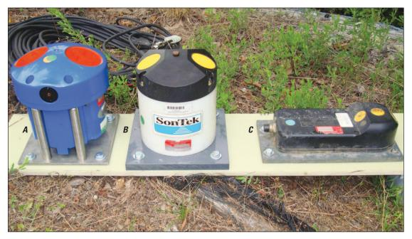
Figure 1. Acoustic doppler current profilers operating at frequencies of (A) 1.2 megahertz, (B) 1.5 megahertz, and (C) 3.0 megahertz.
