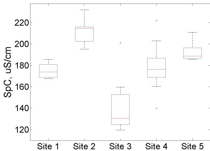
Figure 5. Longitudinal specific conductivity values along Tanyard Creek from upstream to downstream.
