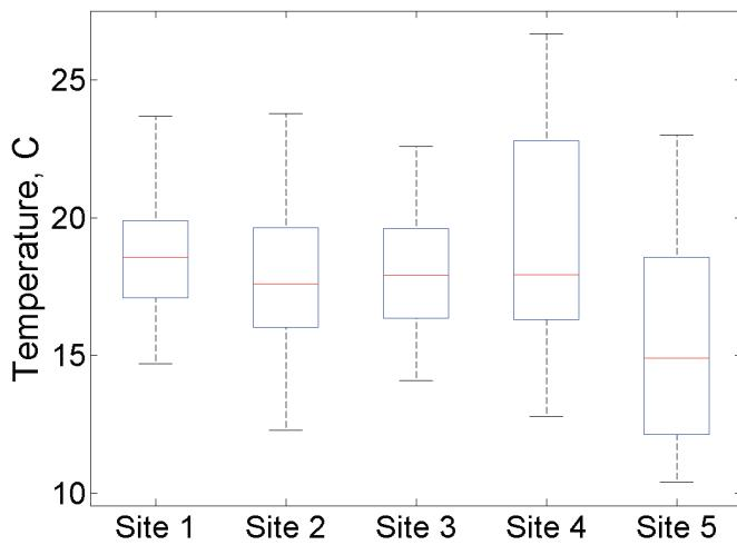
Figure 6. Longitudinal temperature values along Tanyard Creek from upstream to downstream.
