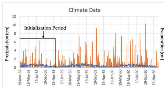
Figure 1. Climate data for HYDRUS 2D model. Precipitation (orange) and evapotranspiration (blue) from March 1958 to December 1960. Initialization of ~270 days was used before simulation with additional two years thereafter. Years 1959 and 1960 were chosen due to the high precipitation events to allow for increased interflow.
