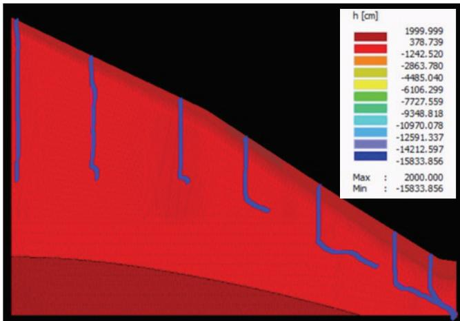
Figure 2. Resulting pressure head at the end of the simulation for a homogeneous soil profile, all other parameters beside soil material are identical for the uniform and non-uniform depth to argillic horizon model. The pathways shown by the particle tracker (blue lines) illustrates the soil water movement when unaffected by soil layering. This figure has been stretched with a ratio of 1 unit vertical to 4 units horizontal to visualize the particle tracking.
