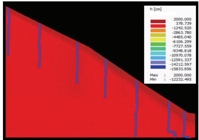
Figure 3: Resulting pressure head for non-uniform depth to argillic horizon hillslope for a simulation of 870 days. The pathways shown by the particle tracker (blue lines) illustrates the soil water movement affected by a thin argillic horizon. This figure has been stretched with a ratio of 1 unit vertical to 4 units horizontal to visualize the particle tracking.
