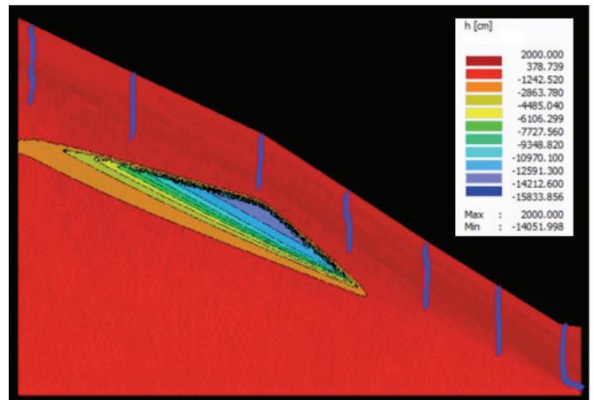
Figure 4: Resulting pressure head for uniform depth to argillic horizon hillslope for a simulation of 600 days. The pathways shown by the particle tracker (blue lines) illustrates the soil water movement affected by a thick argillic horizon. This figure has been stretched with a ratio of 1 unit vertical to 4 units horizontal to visualize the particle tracking.
