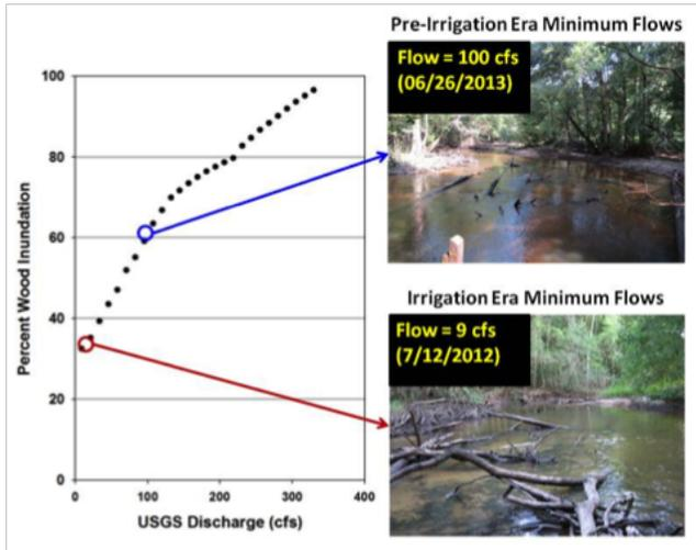
Figure 5: An example of a discharge-inundation relationship for coarse woody material in the stream channel. See Figure 3 for picture details.
