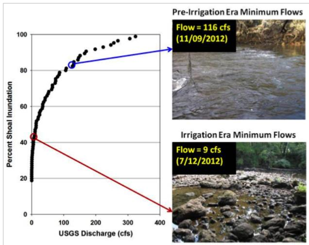
Figure 3: An example of a discharge-inundation relationship for a shoal. Pictures at right show degree of habitat inundation at discharges similar to minimum flows during the pre-irrigation and irrigation periods of record.
