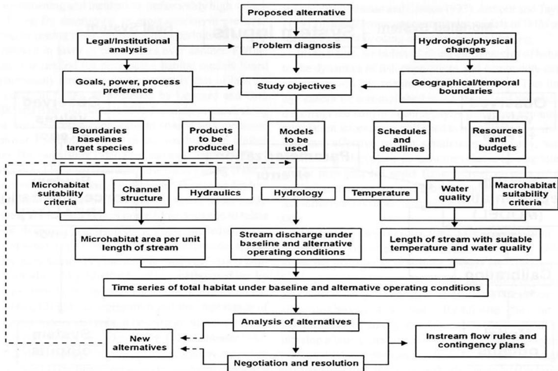
Figure 1. Schematic diagram of the Instream Flow Incremental Methodology (from Bovee et al. 1998).
