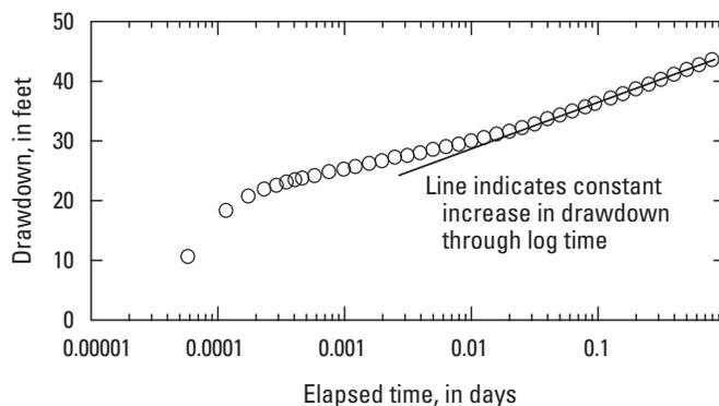
**Figure 3. Drawdown as a function of log time in well 33P030 at a pumping rate of 552 gallons per minute, Fort Stewart, Georgia, April 26, 2010.**
