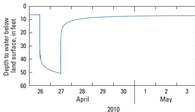
**Figure 4. Measured water level in well 33P030 during a 24-hour aquifer test, Fort Stewart, Georgia, April 26–May 3, 2010.**
