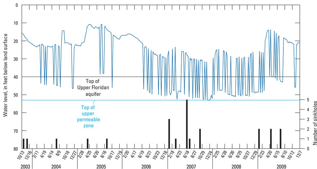
**Figure 3. Water-level measurements in well 12L382 with respect to depth to the top of the Upper Floridan aquifer and the top of the upper permeable zone and number of sinkholes reported during October 2003–December 2009. See Figure 4 for well location.**
