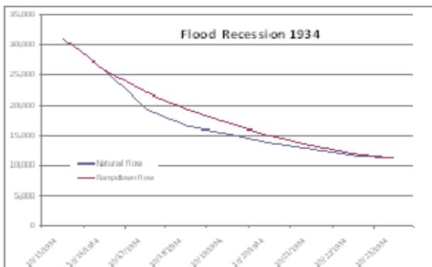
Figure 4. The receding phase of an October 1934 flood and what would happen under the RIOP ramp down control
