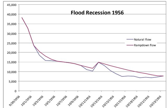
Figure 5. The receding phase of an October 1956 flood and what would happen under the RIOP ramp down control
