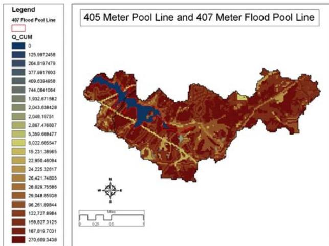
**Figure 8: Map of proposed Peck's Mill reservoir showing the dam site and impounding area for 405 m pool line and 407 m flood pool line.**
