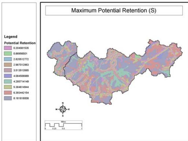
**Figure 5: The maximum potential retention (S) raster for the Peck's Mill Watershed.**
