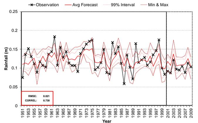
**Figure 2: Inter-comparison between observed winter rainfall time series and ensemble forecastings. Data prior to 2000 are used for model calibration. Data after**
