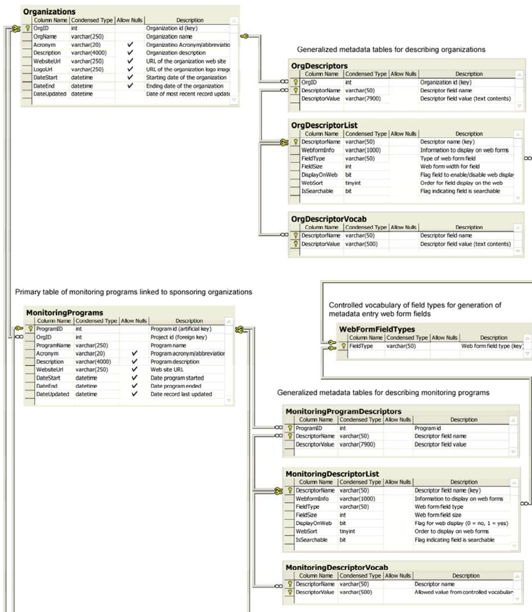
Figure 1. Entity-relationship diagram for organization and monitoring program elements of the NPS\_WaterQuality database (version 1.0). Note that lines represent relationships between tables, with cardinality indicated by a key symbol for the primary table key and infinity symbol for the foreign table
