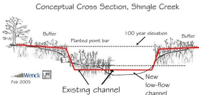
**Figure 6. Desirable stream cross section with enhanced habitat and a low-flow channel.**
