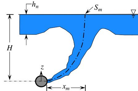
Figure 7. Definition diagram for horizontal buoyant jets
