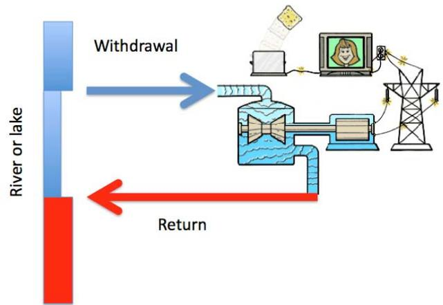
**Figure 2. Thermoelectric power production facility with single-pass cooling water returned to stream. No consumptive use, but water quality is impaired.**
