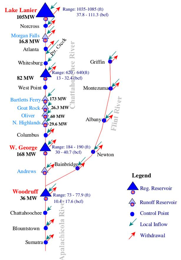
**Figure 1.** ACF basin schematic with indicated components of regulated reservoirs, runoff reservoirs, interested river control point, local inflows, and withdrawals. Installed hydropower capacities are shown in Megawatts (MW). The elevation and storage ranges of regulated reservoirs are shown in feet (ft) and billion cubic feet (bcf).
