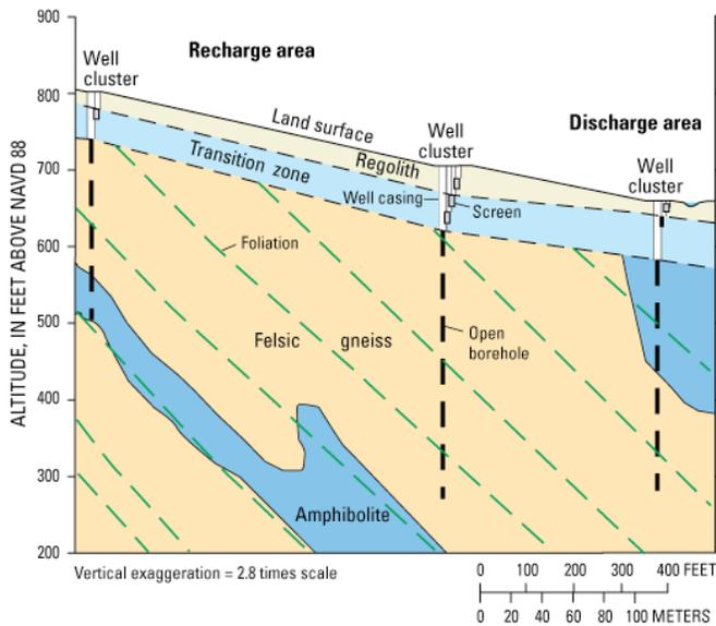
**Figure 2. Typical North Carolina Piedmont and Mountains Resource Evaluation Program research station construction along a topographic transect. The dip-slope transect at the Upper Piedmont research station is shown (NAVD 88, North American Vertical Datum of 1988).**
