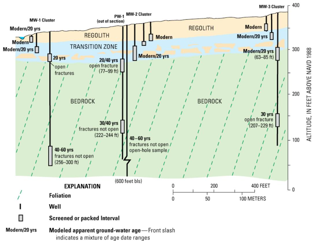
**Figure 5. Overall apparent age interpretations for ground-water samples collected from different zones along a topographic transect (Lake Wheeler Road research station, North Carolina).**
