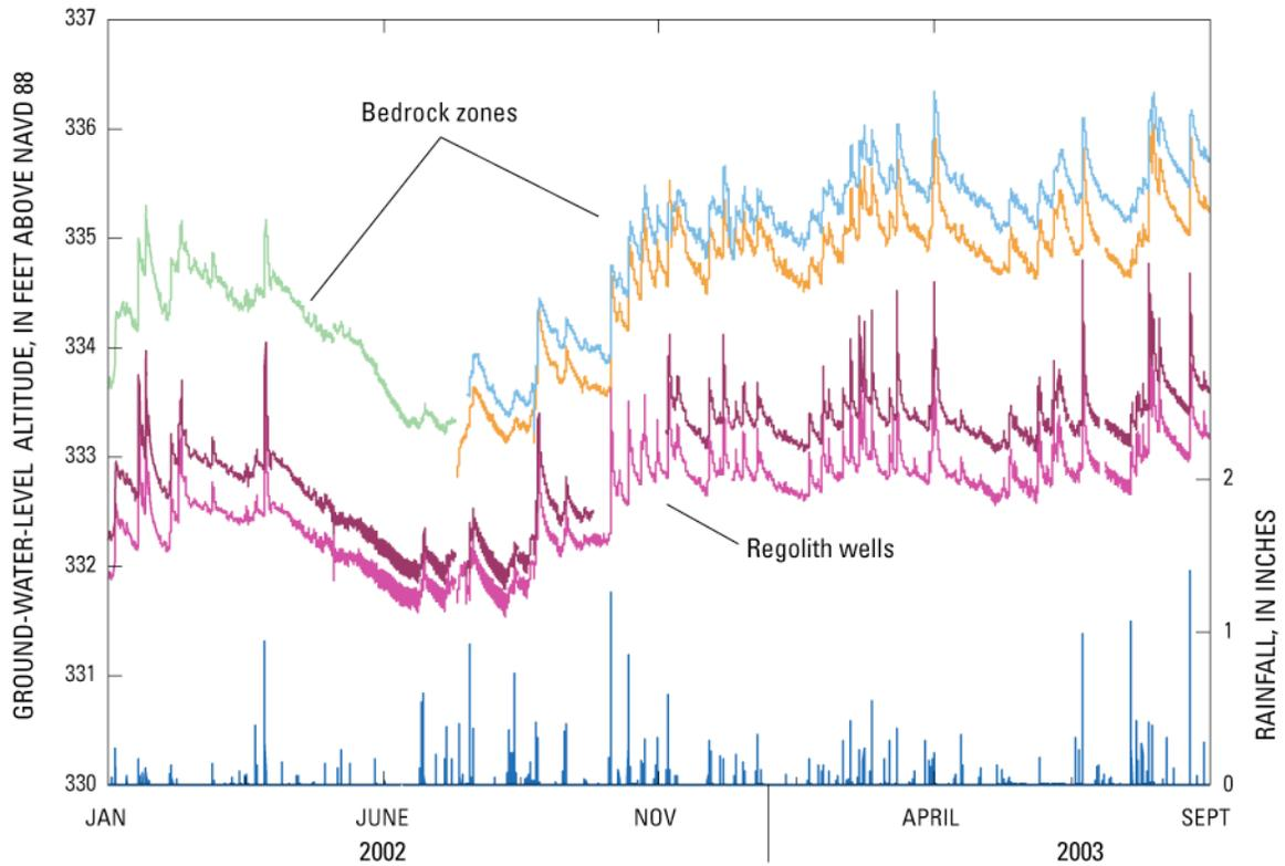
**Figure 4. Continuous ground-water levels recorded in a discharge area at the Lake Wheeler Road research station, North Carolina (NAVD 88, North American Vertical Datum of 1988).**
