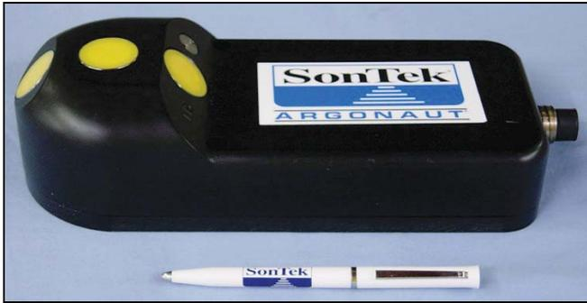
**Figure 2. SonTek® Argonaut–Shallow Water velocity meter; pen for scale.**
