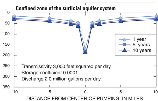
**Figure 3. Estimated drawdown in the lower Brunswick aquifer at a pumping rate of 2 million gallons per day for 1-, 5-, and 10-year time intervals, Camden County, Georgia. See Figure 1 for line of section.**
