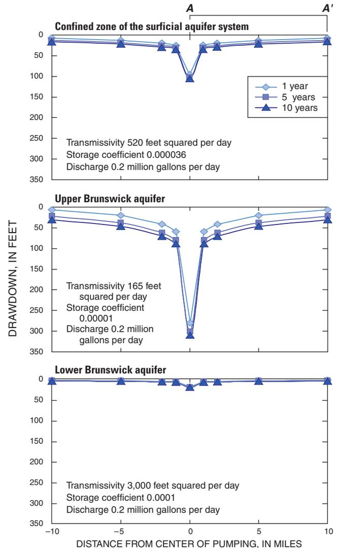
**Figure 2. Estimated drawdown in the confined zone of the surficial aquifer system and in the upper and lower Brunswick aquifers at a pumping rate of 0.2 million gallons per day for 1-, 5-, and 10-year time intervals, Camden County, Georgia. See Figure 1 for line of section.**
