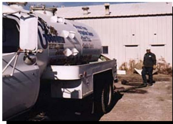
Photo1. Septage handler discharges at WWTP.
