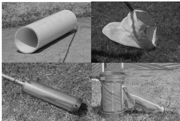
**Figure 1. Sampling devices used (clockwise from top left): large corer, D-frame sweep net, Hess sampler, Ogeechee corer.**
