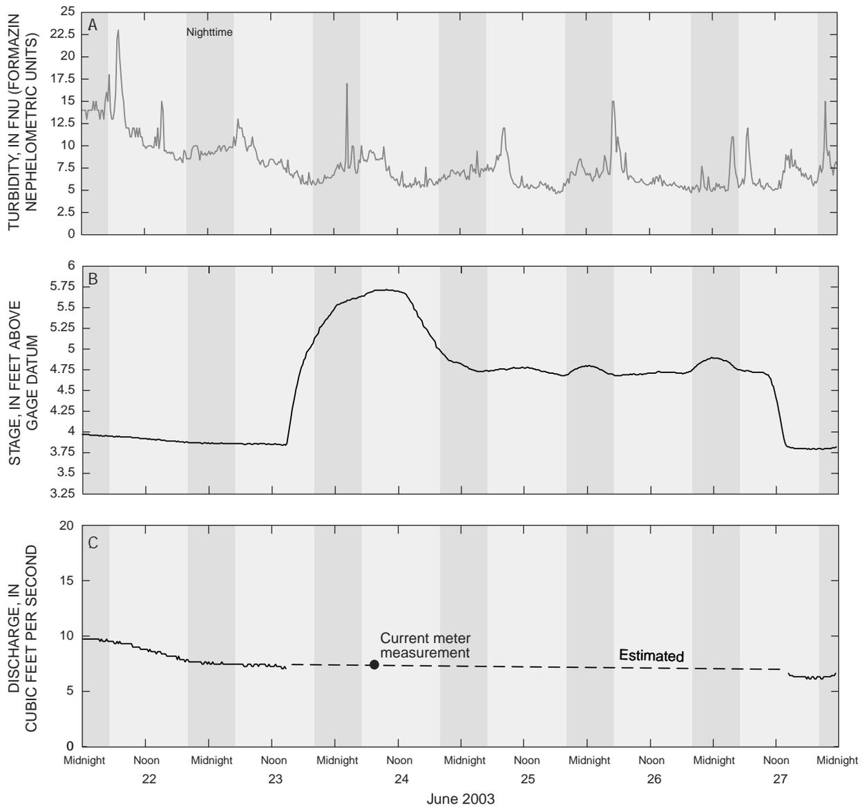
**Figure 2. Turbidity, stage, and discharge data for Crooked Creek near Norcross, Georgia June 22–27, 2003.**
