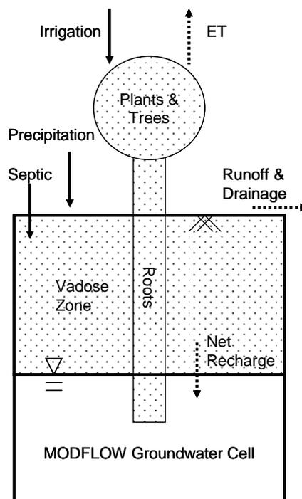
**Figure 1. Conceptual diagram of a cell in the SV Package. The filled areas (vadose zone, plants/trees, roots) are part of the SV Package domain. Solid arrows indicate specified inflows. Dotted arrows indicate computed outflows.**
