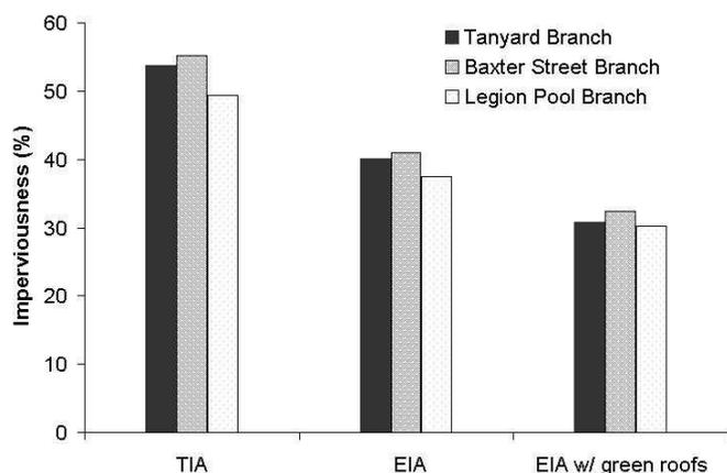
**Figure 4: Total Impervious Area (TIA) and Effective Impervious Area (EIA) for three watersheds.**
