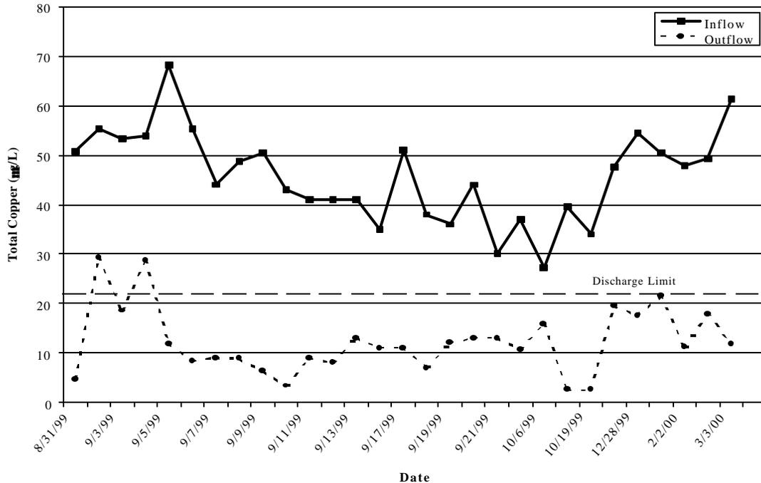
**Fig. 2. Total recoverable copper in inflow and outflow water from a physical model constructed wetland system.**
