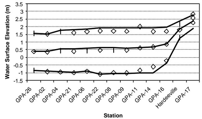
**Figure 4. Measured (diamonds) and simulated (solid lines) water surface elevation percentile comparisons (5th, 50th and 95th) along Front River.**
