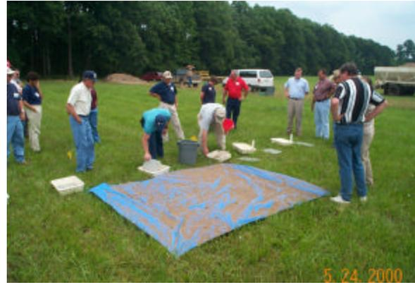
**Figure 4. Poultry litter spreader calibration.**
