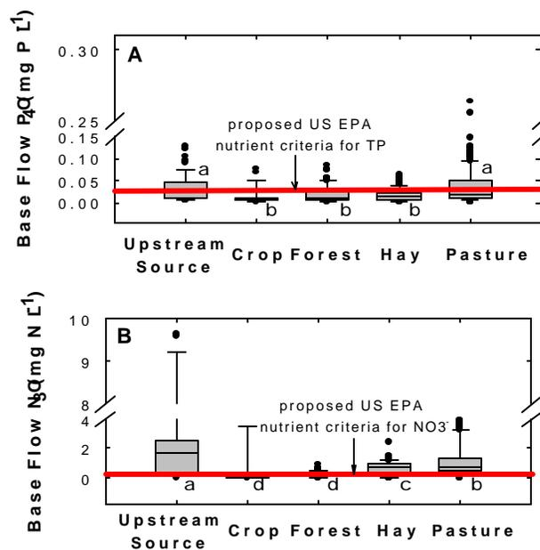
**Figure 2.** Boxplots of dissolved reactive phosphorus (A) and nitrate (B) for management systems. Center line in each boxplot marks the median value. Upstream source management system indicates rural housing. Unlike lower case letters indicate medians are significantly different (Fisher's LSD,  $p < 0.05$ ). Note US EPA nutrient criteria are for Ecoregion IX.
