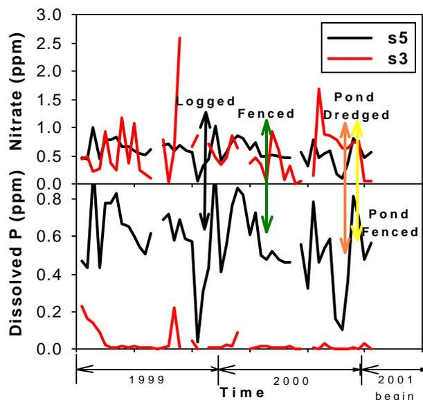
**Figure 5. Stream base flow nitrate (upper) and DRP (lower) concentrations from December, 1998 to January, 2001. Note that stream site s5 is coming into pond and s3 is exiting the pond.**
