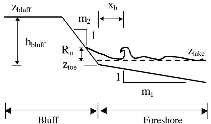
**Figure 1. Simplified geometry of shoreline. Parameters defined in Table 1.**
