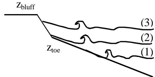
**Figure 2. Cases considered for erosion prediction methodology. Case (1): mean water level is below the toe of the bluff, and runup does not rise above the toe of the bluff. Case (2): mean water level is below the toe of the bluff, but the runup rises above the toe of the bluff. Case (3): mean water level is above the toe of the bluff.**
