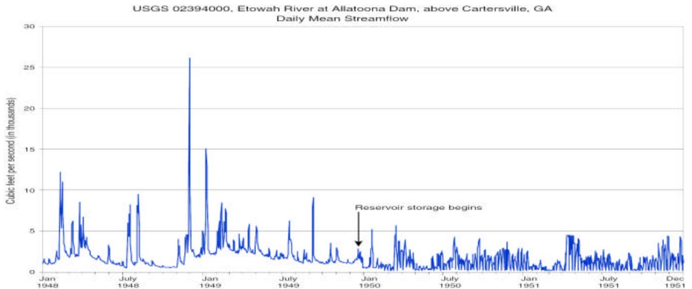
**Figure 1. Streamflow fluctuations before and after construction of Allatoona Dam on the Etowah River.**
