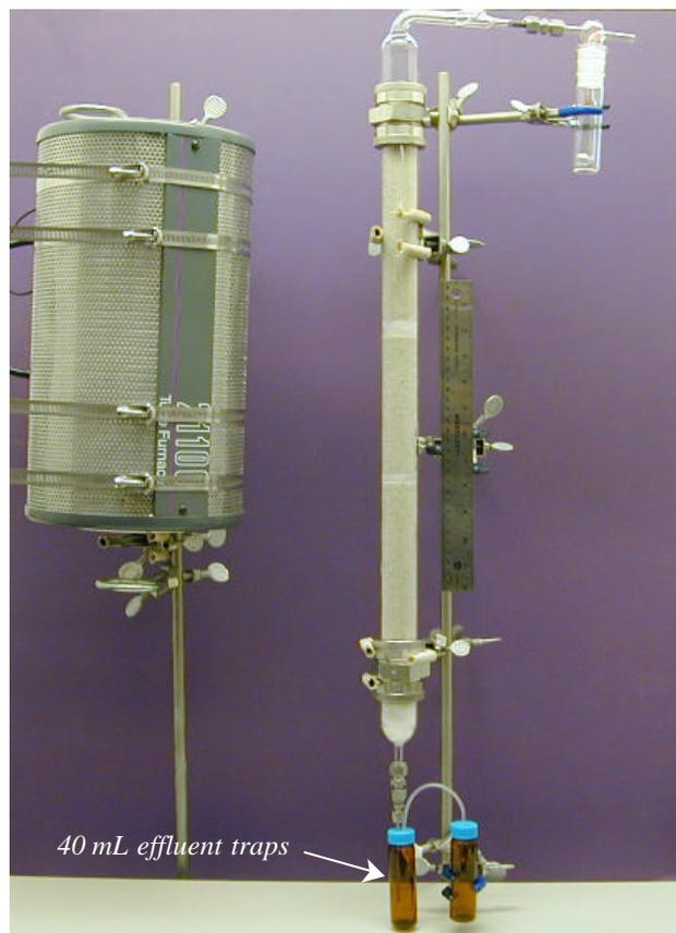
**Figure 1. Tube oven and sand-filled quartz tube reactor.**
